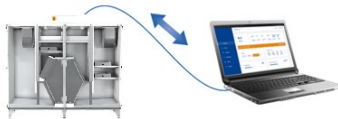
Ventilation unit is connected to a computer by cable via ethernet interface
